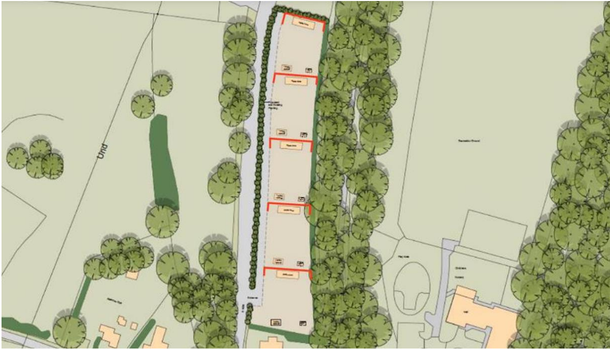
Figure LA5: Extract from WS Planning and Architecture Drwg No: J004472-DD-05 Rev A. The red line shows the proposed position of the 2.3m high acoustic noise fence (taken from Noise assessment Report 1510.NIA.00) (CD1.22)
