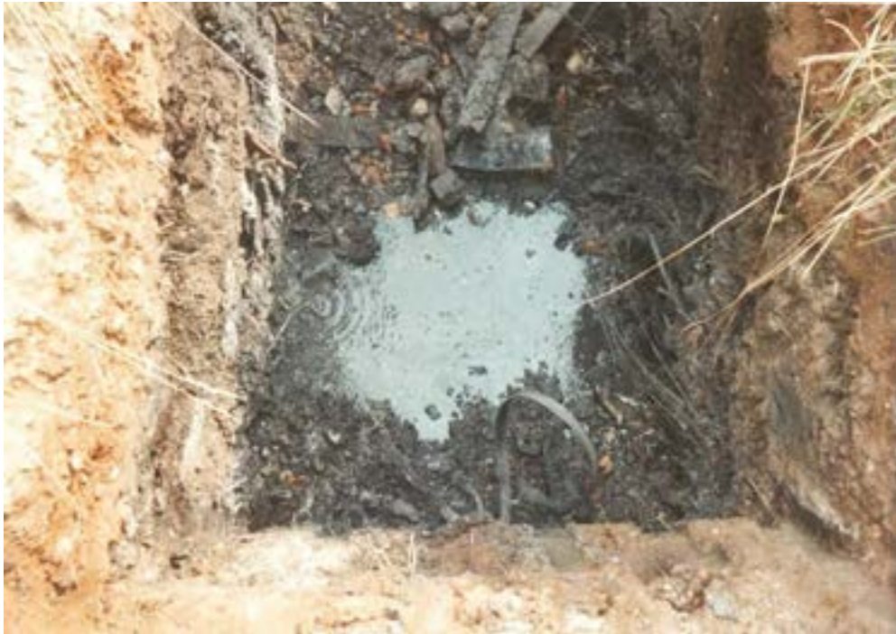
Plate 4. Leachate Seepage at 1.8m with gas emission
