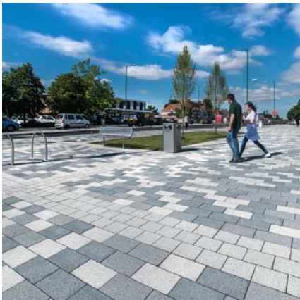
To building entrances and footpaths within plots Granite concrete paving blocks, preferably permeable: e.g. Fusion by Tobermore (image copyright Tobermore)
