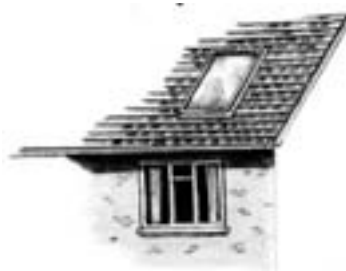
If headroom allows, rooflights are less obtrusive
