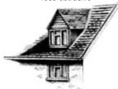
Acceptable dormer that is set into the roof and matches the windows below
