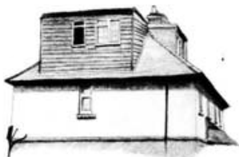
A large flat-roofed dormer that dominates the house and perhaps next door as well
